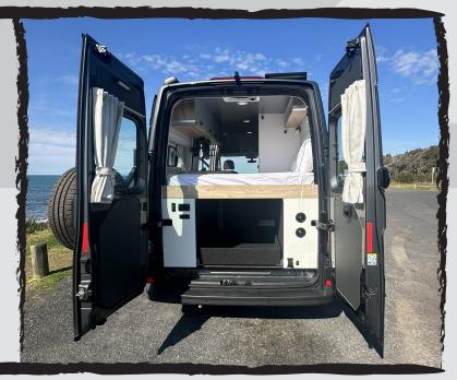
This van has ample storage in the galley & overheads. The east/ west bed allows for more internal space within the van. Under the bed is your power & hot water system at each end. Standard open space under bed & options for different under bed configurations.
